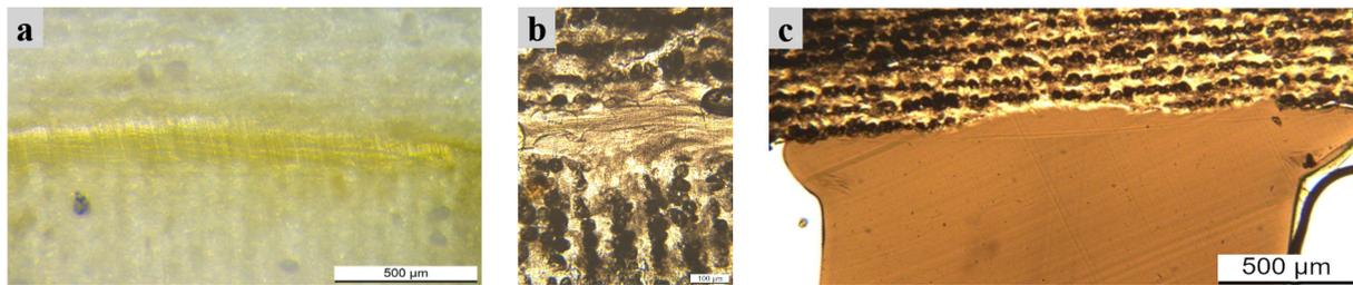
Fig. 5. (a) reflection microscope image of a cross section of the weld seam (AM-AM); (b) thin section of the weld seam (AM-AM); (c) thin section of the weld seam (AM-IM)
