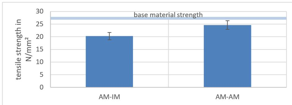
Fig. 4. Tensile strength of welded AM-IM and AM-AM parts in relation to AM base material strength, n = 3
