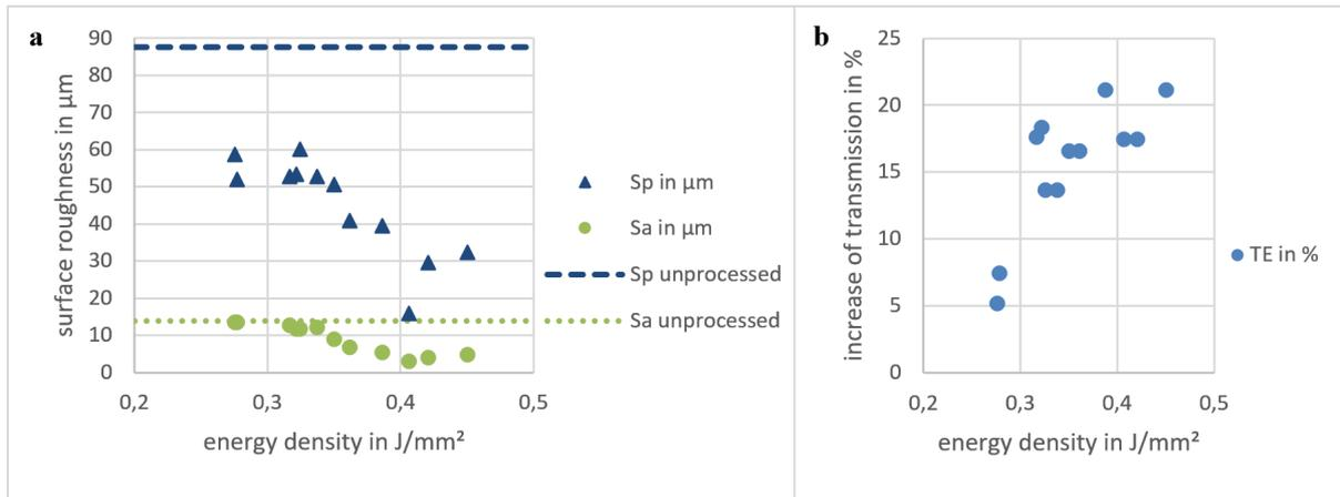
Fig. 2. (a) surface roughness,  $S_a$  - arithmetic mean roughness and  $S_p$  - maximum profile peak height and (b) increase of transmission as a function of introduced energy density
