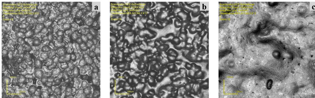
Fig. 3. Laser scanning image of (a) the unprocessed surface; (b) the surface after irradiation with  $0.317 \text{ J}/\text{mm}^2$ ; (c) the surface after irradiation with  $0.450 \text{ J}/\text{mm}^2$
