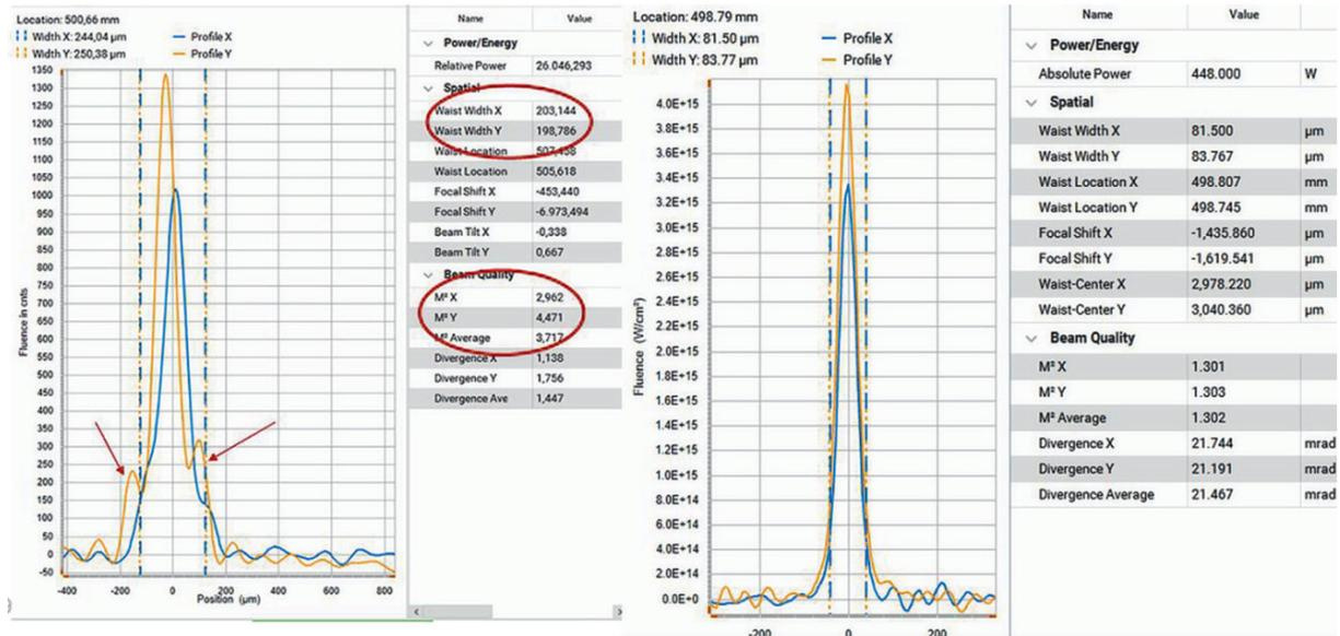
Fig. 4. Measurements on an SLM system at the Fraunhofer IAPT: On the left the laser system with quality problems, on the right the laser system with perfect results (©Fraunhofer IAPT)
