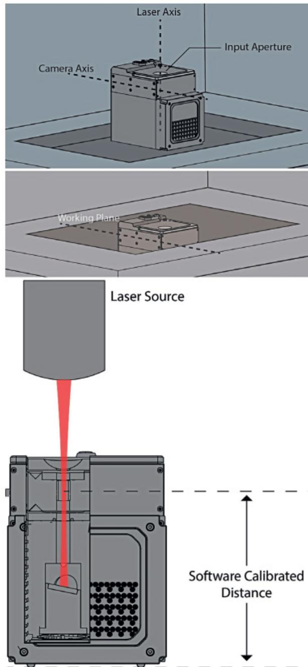
Fig. 3. Measuring principle and application of non-contact beam measurement.
