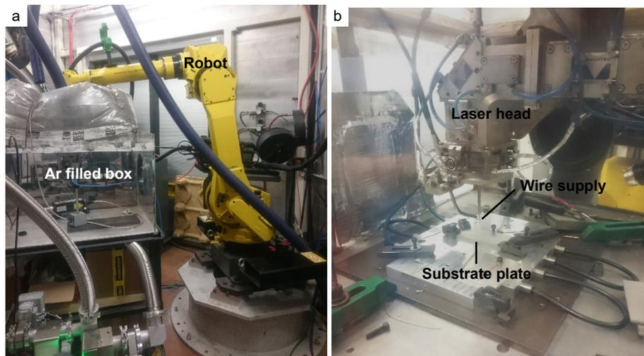
Fig. 1. Experimental setup: (a) external and (b) internal view.
