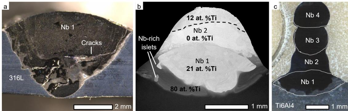
Fig. 2. (a) Typical niobium cladding on 316L plate ( $V = 0.1$  m/min), (b) SEM image of two niobium layers cladded on Ti6Al4V plate, (c) four niobium layers cladded on Ti6Al4V plate.
