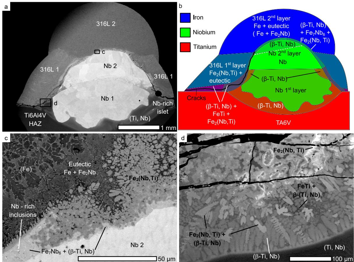
Fig. 3. Crosscut of cladded 316L/Nb/Ti6Al4V assembly: (a) general SEM view; (b) mapping of the mixing processes based on X-map and EDS; (c) reactive layer between 316L 2 and Nb 2 clads; (d) reactive layer between Ti-rich melt formed during niobium cladding and 316L 1.
