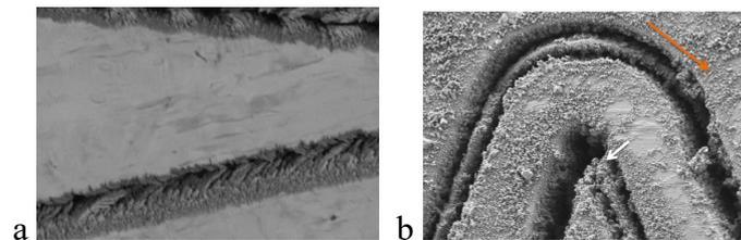
Fig. 2. Experimental observations in stent cutting (a) Top-view of feather-like structures on the cutting edge (b) Top-view of "Dust-Blade" inside the cutting kerf (marked by white arrow) and debris on the workpiece surface (marked by orange arrow)
