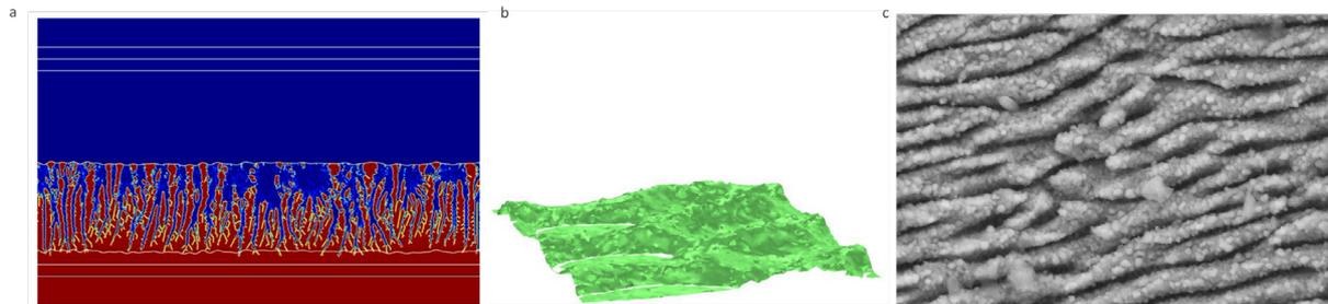
Fig. 6. (a) Simulation result of ripple formation in a 2D cross-section, in red color the bulk material that was not ablated, in blue the void area, white lines show different locations in the simulation domain (initial surface, PML area, sender line); (b) Simulation result of ripple formation in 3D; (c) Actual ripple structures in photographic measurement (from Zhu Liu (2019)).
