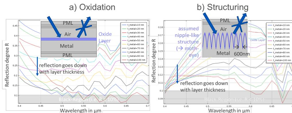
Fig. 5. There are two different mechanisms (analyzed on the left and right), by which the blackening effect in black marking is achieved:
