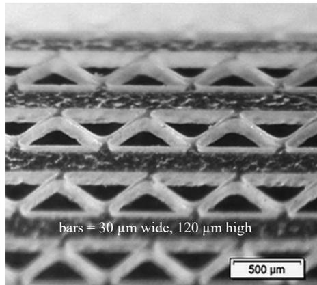
Fig. 6. Microscope image of fs laser cut sample geometry in PDLLA sheet.
