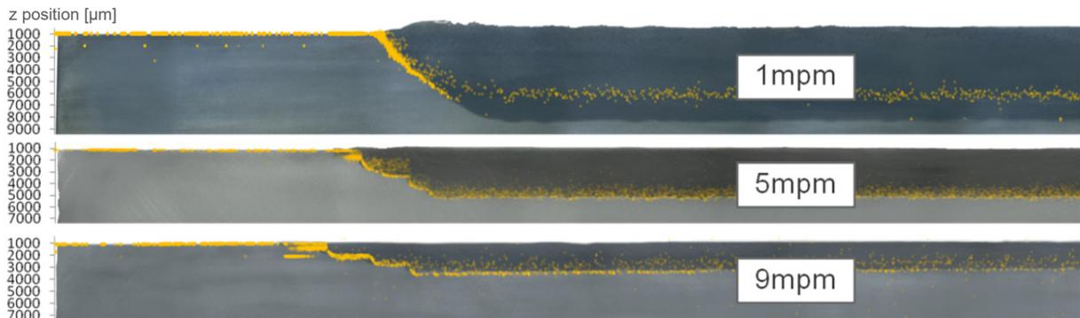
Fig. 1. Cross-section pictures and interferometer data (yellow points) at different feed rates. The workpiece surface was positioned at 1000  $\mu\text{m}$  offset to achieve a safe reference for data collection even after a possible material deformation.
