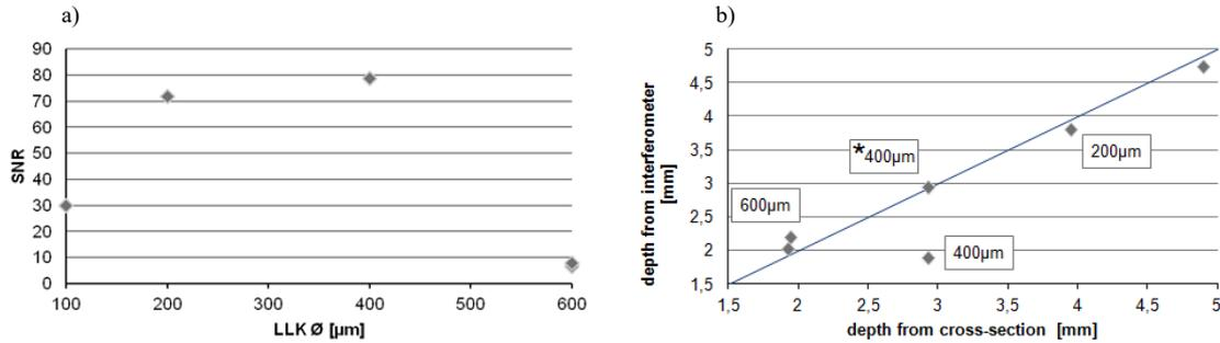
Fig. 5. a) Signal to noise ratio, and b) depth from the interferometer versus depth from the cross-sections.
