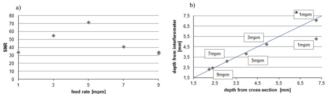
Fig. 3. a) Signal to noise ratio, and b) depth from the interferometer versus depth from the cross-sections.
