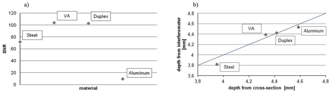
Fig. 6. a) Signal to noise ratio, and b) depth from the interferometer versus depth from the cross-sections.
