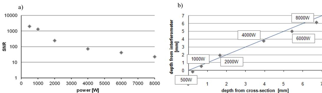
Fig. 4. a) Signal to noise ratio, and b) depth from the interferometer versus depth from the cross-sections.
