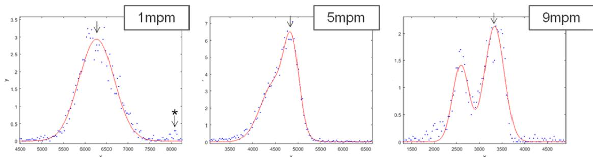
Fig. 2. Gaussian fits of the noise corrected interferometer data. The arrows mark the highest peak that has been used to determine the capillary depth.
