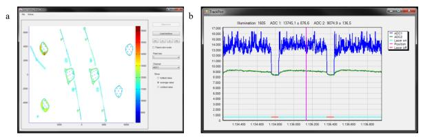
Fig. 2. (a) Layerwise x/y 2D representation of thermal emissions; (b) Complementary Track Plot of selected scan vector.
