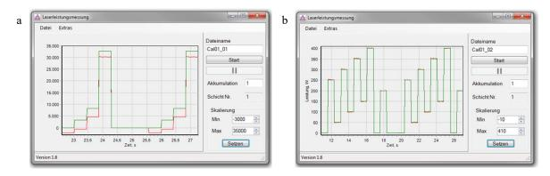
Fig. 3. (a) Adjustment for set and measured laser power; (b) Calibration rechecks for laser power adjustment up to 400 W.
