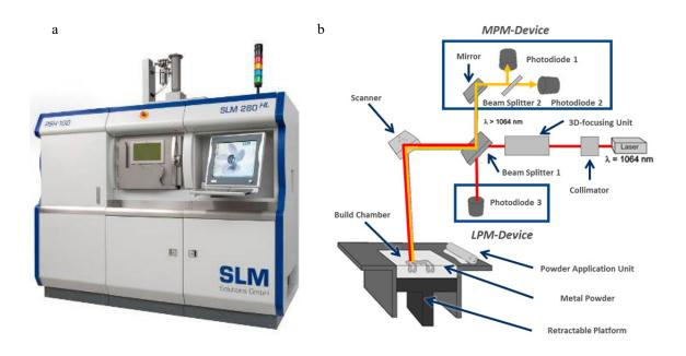
Fig. 1. (a) SLM 280<sup>HL</sup>; (b) Schematic assembly of optic design with Melt Pool Monitoring and Laser Power Monitoring.
